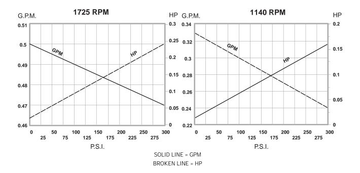
BSM Pump Corp. - MANUFACTURING SOLUTIONS TO PUMPING PROBLEMS FOR OVER 100 YEARS.
